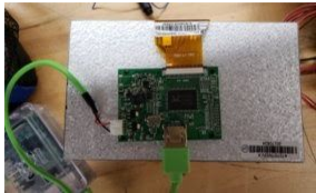
Fig. 6 Back side of the LCD Display used for the touch free eye tracking headset
